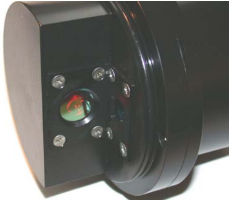
Fig. 3 Optical part of measuring-head after removing cover of flow-through chamber; the excitation window (right hand side) and detector window (left hand side) form a right angle with each other and are in vertical position in order to minimize deposit of phytoplankton.
