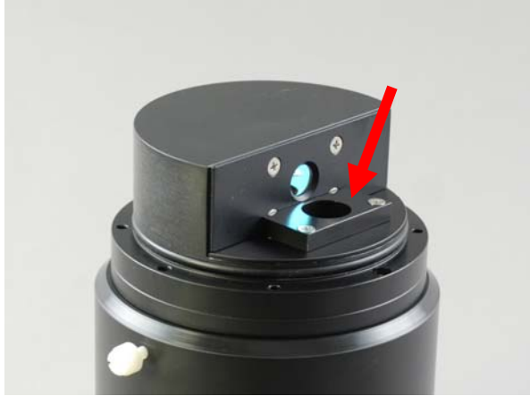
Fig. 6 here the cuvette holder frame is already mounted on the WATER-FT head. The small plastic part holds the sample cuvette WATER-K in place during the measurement. The part is fixed with two long screws that replace the shorter ones used on this position in the default head.
