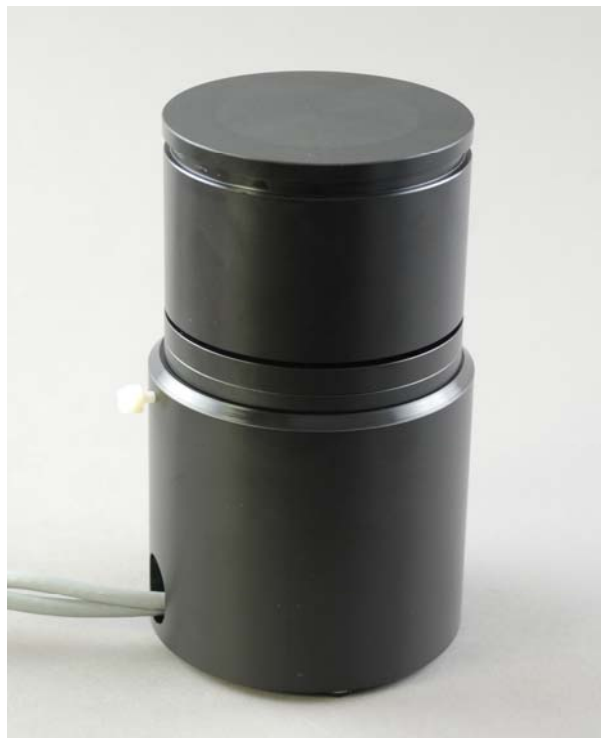
Fig. 7 the housing is closed with the second tube and a separate lid to prevent ambient stray light to illuminate the sample. Now the WATER-FT head can be used upright with a round cuvette.
