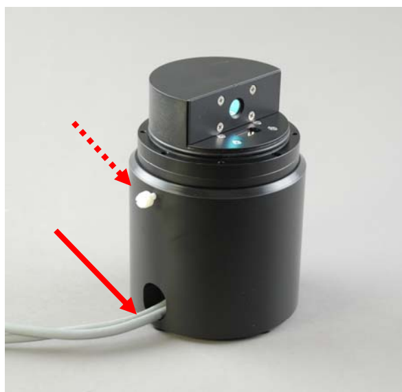
Fig. 5 shows the WATER-FT head mounted on the base of WATER-FT/S. The cables just have to be pulled through the hole in the base tube so that they can be connected with the PAM Control unit. The head itself can just be stuck into the tube from the top and if the white plastic screw (dashed arrow) is tightened, it can not fall out accidentally.
