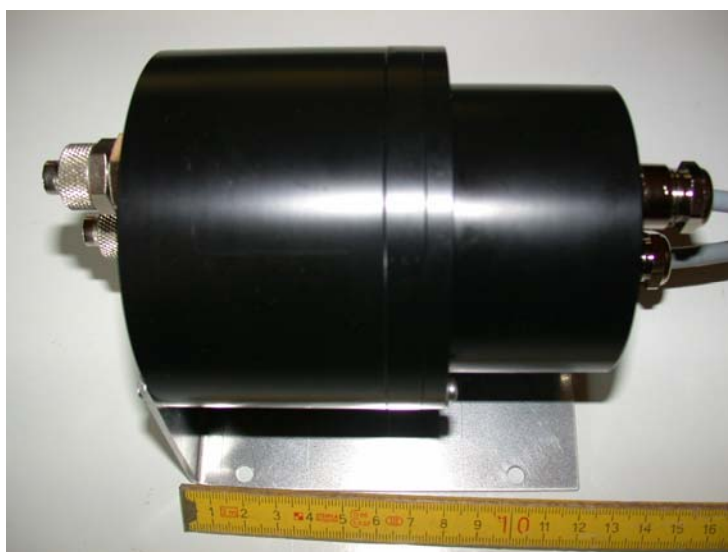
Fig. 1 Measuring-head covered with flow-through chamber, with the water inlets/outlets at the left side and the electrical cables connecting to the PAM-Control unit at the right side. Depicted scale showing centimeters.
